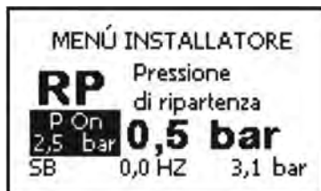
Figure 17: Setting the restart pressure
