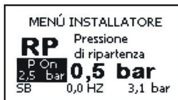
Figure 18: Setting the restart pressure
