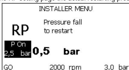
Figure 18.1: Setting the restart pressure (2)
