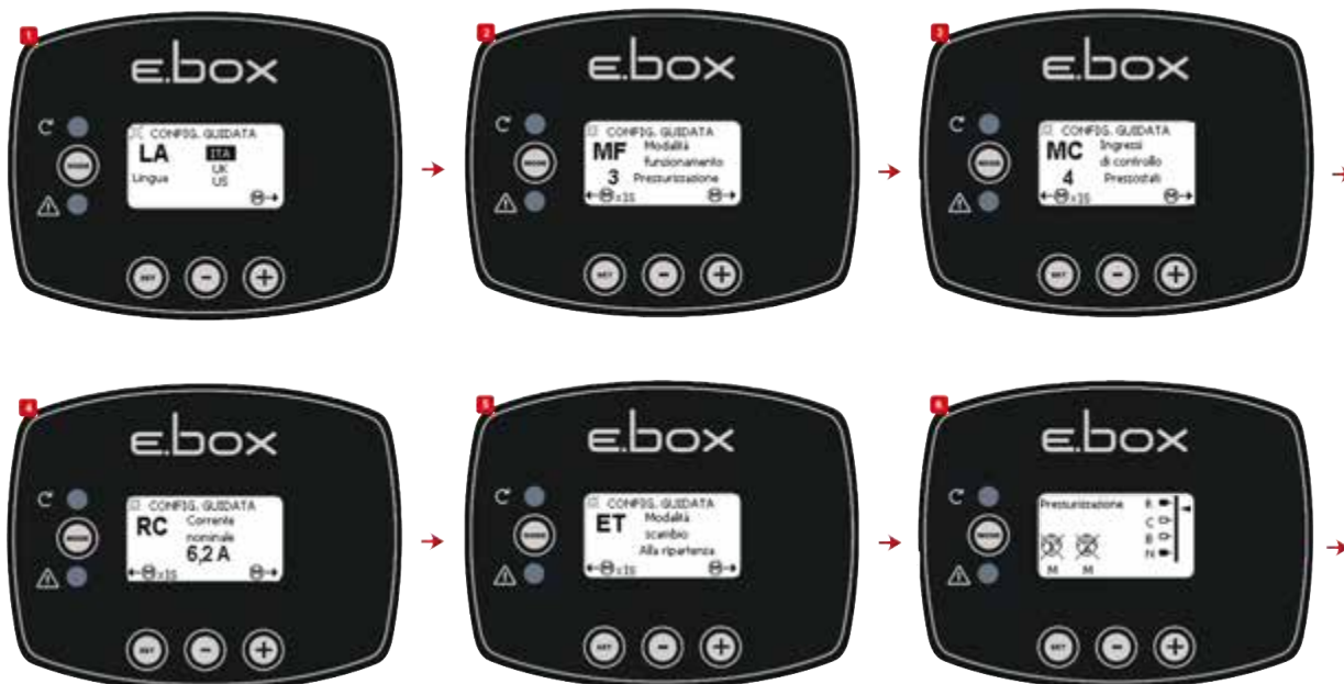
Figure 13: Configuration with pressure switches
