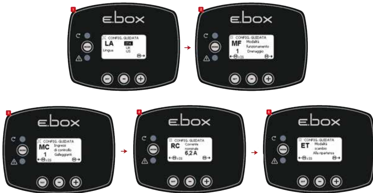
Figure 36: Configuration of Drainage floats or level probes
