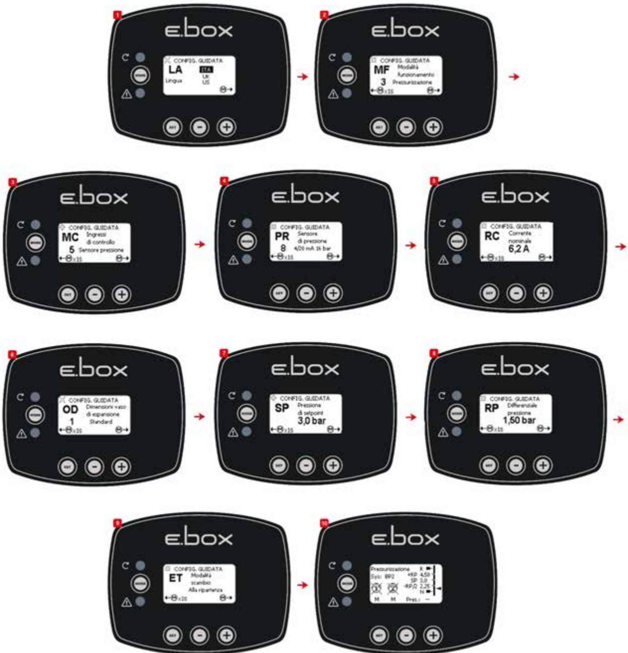
Figure 12: Configuration with a pressure sensor
