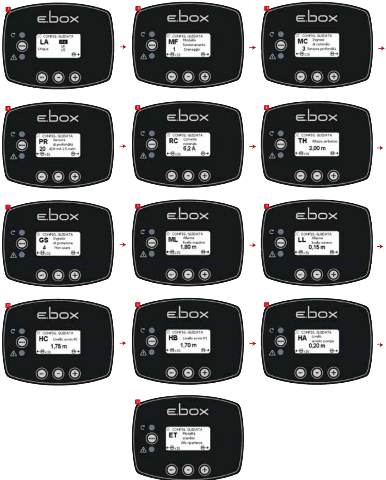
Figure 38: Configuration with only a depth sensor
