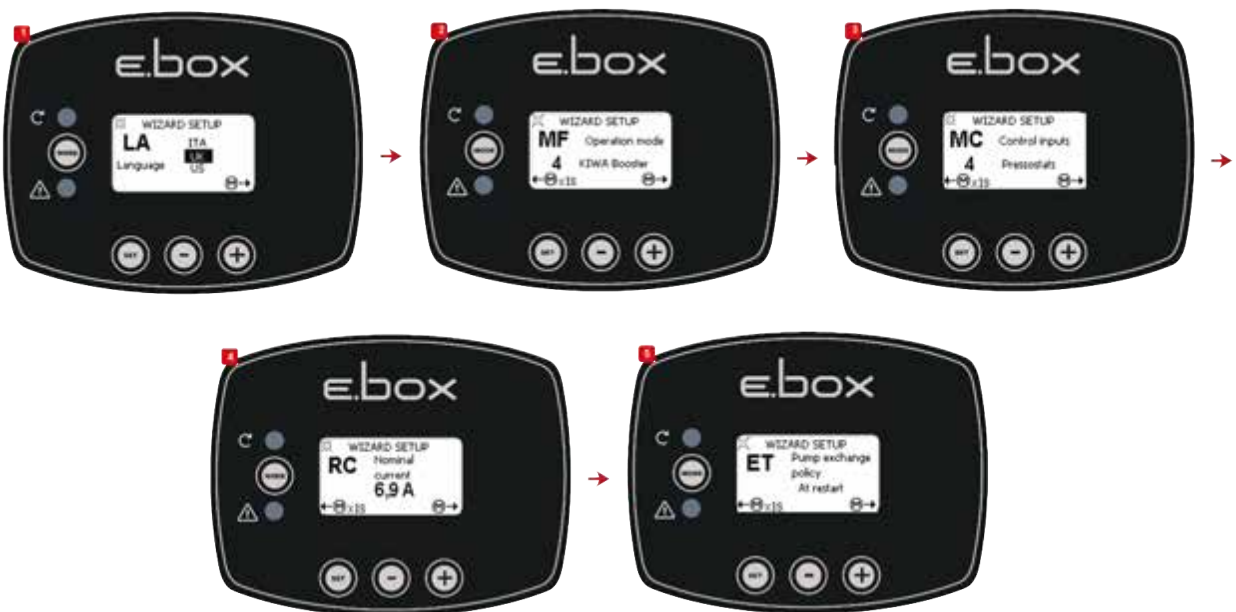
Figure 49: Kiwa configuration with pressure switches
