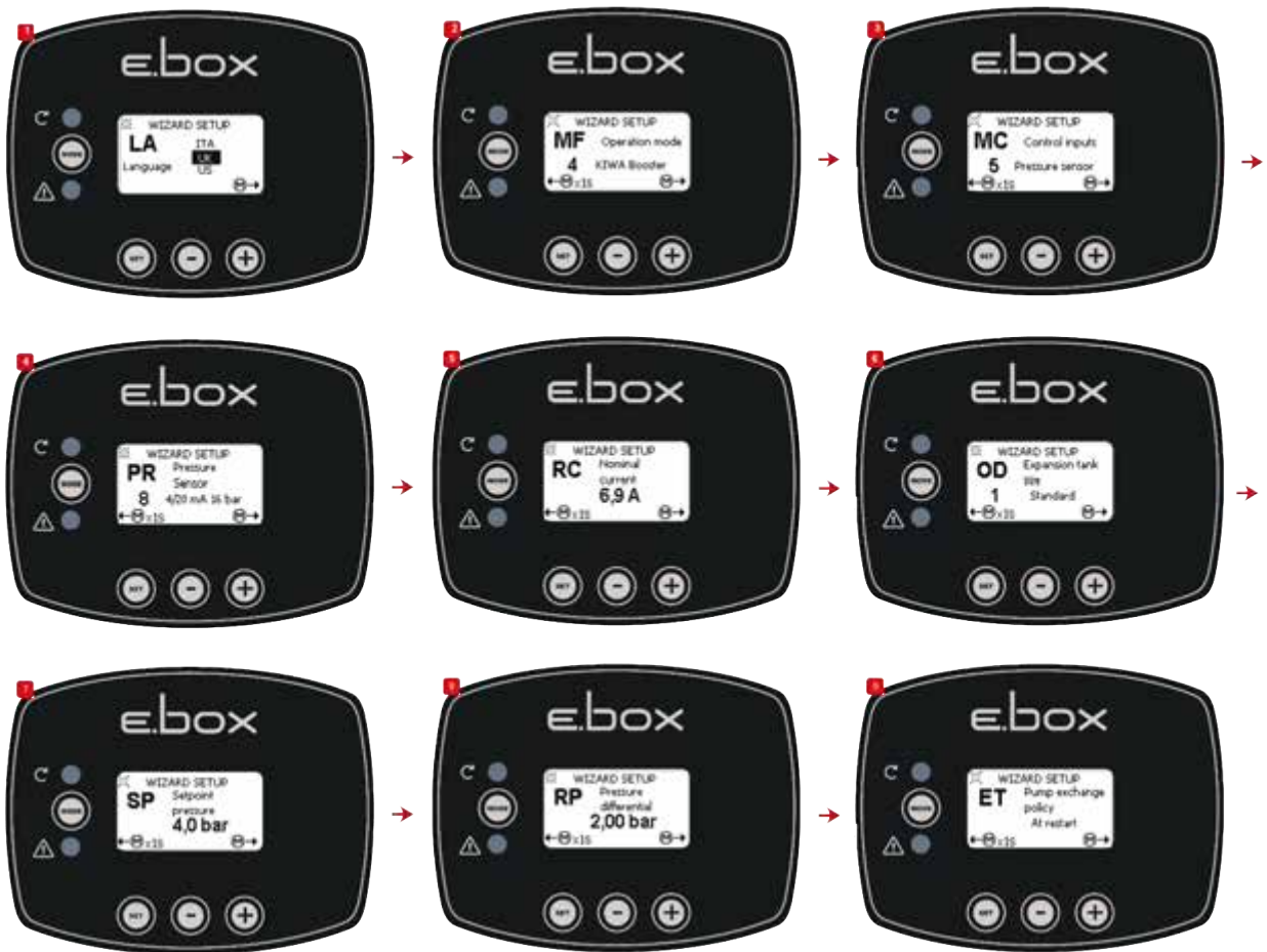
Figure 48: KIWA pressure boosting with pressure sensor
