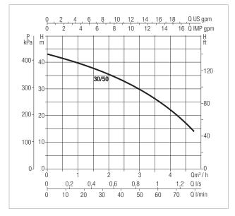
The performance curves are based on the kinematic viscosity values = 1 mm²/s and density equivalent to 1000 kg/m³. Curve tolerance according to ISO 9906.
