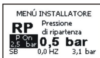
Figure 14: Setting the restart pressure
